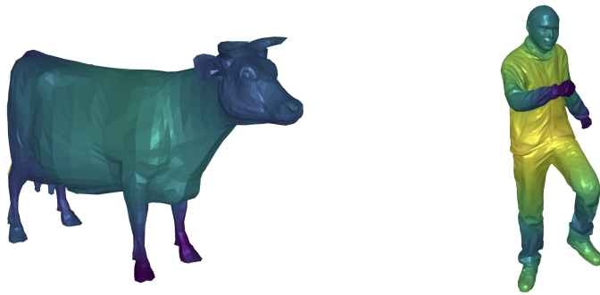
Figure 7: Heat Kernel Signature distance at time interval of [1, 10] Left: Heat Kernel Signature distance on cow.obj Right: Heat Kernel Signature distance on human.obj
